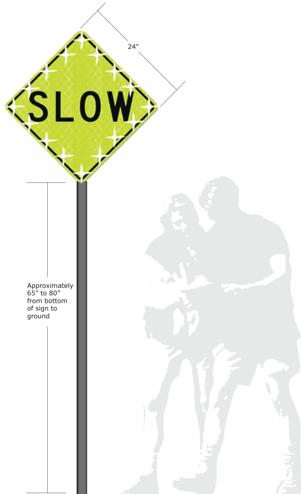
FLASHING SLOW SIGN (SOLAR)
