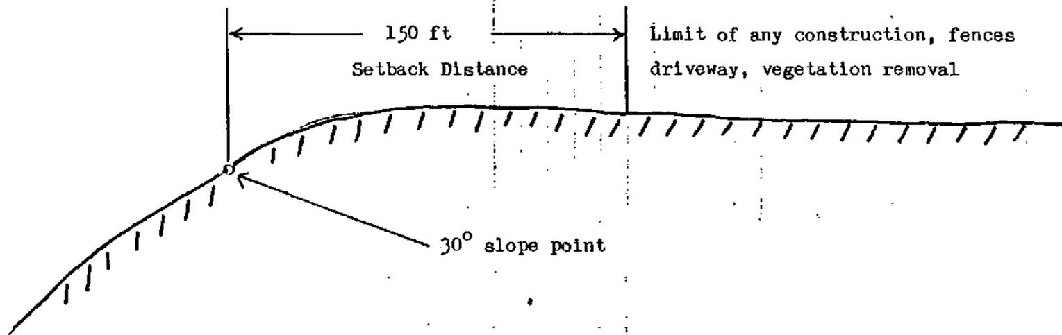
FIGURE 2. Mitigation concept to be used on lots 11 - 19, 38 - 45, and 54 - 56. As discussed in the text, insufficient space may exist on some of the lots for this concept to be executed. Field measurements are necessary to determine the precise location of the 30° point on each lot which would determine the 150 foot setback distance.
